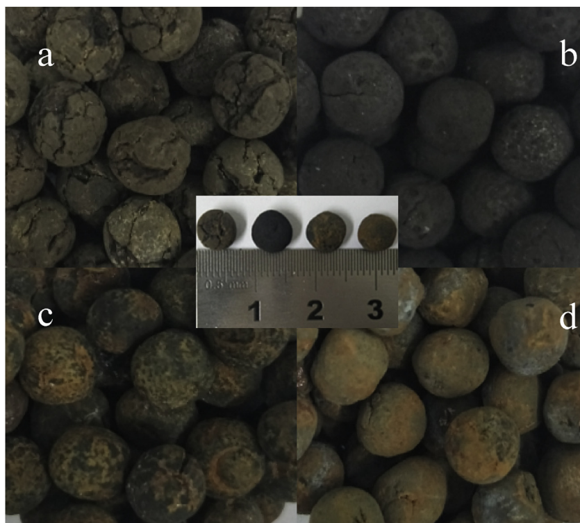
Fig. 1. Images of GSC samples under different carbonization temperature: (a) 300 °C/GSC, (b) 500 °C/GSC, (c) 700 °C/GSC, (d) 900 °C/GSC.
